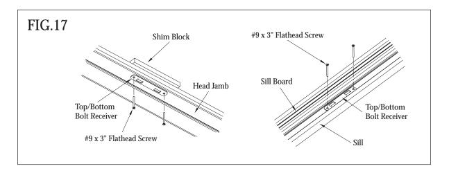
Replace with and fasten the Hook Bolt Receiver and Latch Receiver using #9 x 3" screws. (See Fig.18)
